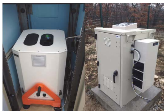
Figure 1. CIMEL CE376 micro-pulse LIDAR set up at Observatoire de Haute Provence (OHP), France
